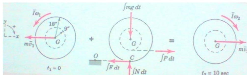
$$[(G_x)_1 + \int_{t_1}^{t_2} \sum F_x dt = (G_x)_2] \Rightarrow \frac{120}{32.2}(-3) + \int_0^{10} (1.5t - F) dt = \frac{120}{32.2} \left[ \frac{18}{12} \omega_2 \right] \quad (\text{I})$$
