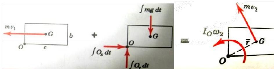
$$(H_O)_1 = mv_1 \frac{b}{2} , \quad H_O = I_O \omega \Rightarrow (H_O)_2 = \left[ \frac{1}{12} m(b^2 + c^2) + m\left(\frac{c}{2}\right)^2 + \left(\frac{b}{2}\right)^2 \right] \omega_2 = \frac{m}{3} (b^2 + c^2) \omega_2 \quad (1) \text{ برخورد}$$
