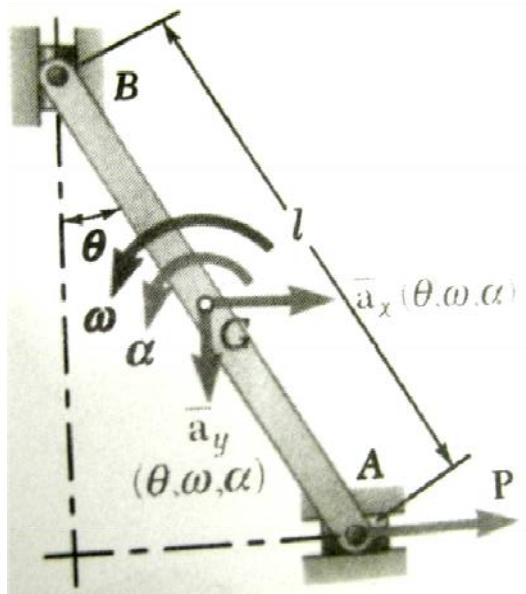
$$\begin{aligned}\vec{a}_B &= \vec{a}_A + \vec{a}_{B/A} \\ a_A &= l\alpha \cos \theta \\ a_B &= l\alpha \sin \theta \\ \vec{a}_G &= \vec{a} = \vec{a}_A + \frac{l}{2} \underbrace{\vec{a}_{G/A}}_{a_{G/A}}\end{aligned}$$
