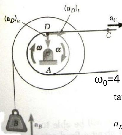
$$v_B = r\omega = (5\text{in})(10 \frac{\text{rad}}{\text{s}}) = 50 \frac{\text{in}}{\text{s}} \Rightarrow v_B = 50 \frac{\text{in}}{\text{s}} \quad \text{(ب)}$$
