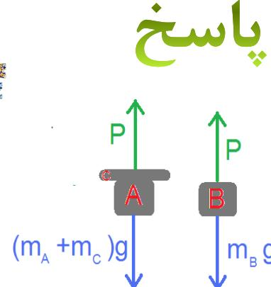
$$\begin{aligned} T_2 &= \frac{1}{2} (m_A + m_B) v_2^2 = \frac{1}{2} (4 + 5)(1.716)^2 = 1325 \text{ J} \\ T_3 &= \frac{1}{2} (9)v_3^2 = 4.5v_3^2 \\ (U_{2 \rightarrow 3})_A &= (4 * 9.81 - P')(1 - 0.3) \\ (U_{2 \rightarrow 3})_B &= (P' - 5 * 9.81)(1 - 0.3) \\ (U_{2 \rightarrow 3})_{Total} &= (-1 * 9.81)(0.7) = T_3 - T_2 \\ v_3 &= 1.19 \text{ m/s} \end{aligned}$$
