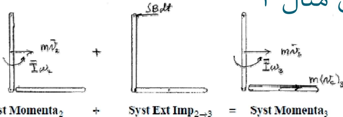
moments about B:  $m\bar{v}_2 \frac{L}{2} + \bar{I}\omega_2 + 0 = m\bar{v}_3 \frac{L}{2} + \bar{I}\omega_3 + m(v_C)_3 L$
