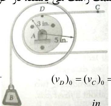
$$(v_D)_0 = (v_C)_0 = 12 \frac{\text{in}}{\text{s}} \rightarrow \quad (a_D)_t = a_C = 9 \frac{\text{in}}{\text{s}^2} \rightarrow \quad \text{(الف)}$$
