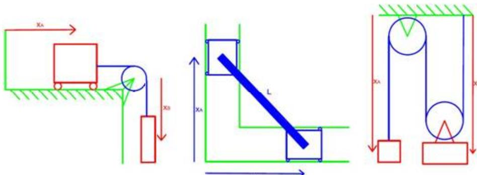
$$\Delta x_A = \Delta x_B \quad \Delta x_A + 2\Delta x_B = \text{Const.} \quad x_A^2 + x_B^2 = L$$
