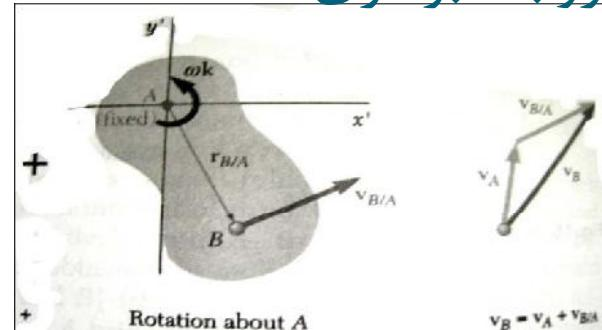
$$\left. \begin{array}{l} \vec{V}_B = \vec{V}_A + \vec{V}_{B/A} \\ \vec{V}_{B/A} = \omega \hat{k} \times \vec{r}_{B/A} \end{array} \right\} \Rightarrow \vec{V}_B = \vec{V}_A + \omega \hat{k} \times \vec{r}_{B/A}$$
